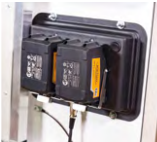
2 light weight Li-Ion batteries mounted on the machine
